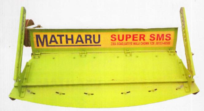
MATHARU SUPER SMS, FITTED ON VISHAL-435 BRISK SELF PROPELLED COMBINE HARVESTER
